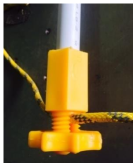
Dropper Connection With Rope
